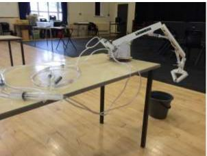
Students work in small groups with a volunteer to make a crane or robotic hydraulic arm from card, syringes and plastic tubing. They will also see demonstrations of modern lifting and accessing equipment and go up and operate the historic Cargo Cranes.
